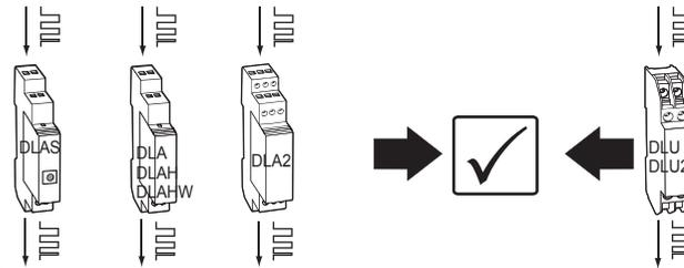
Line still on in case of removal plug-in module :
