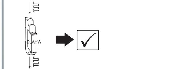
Line cut-off in case of removal of plug-in module :
